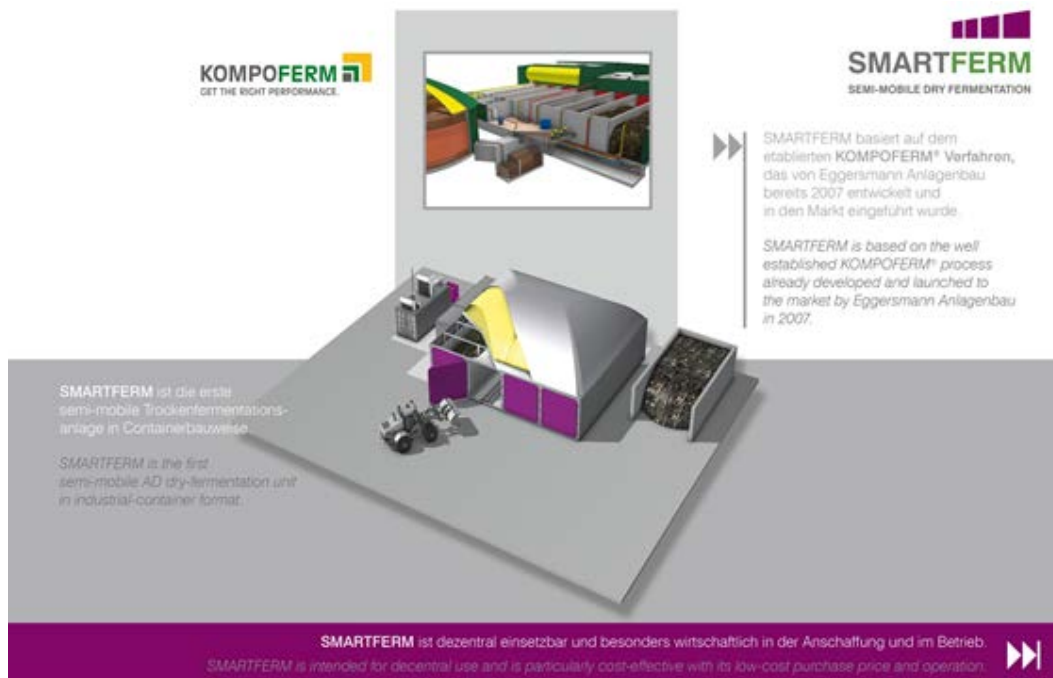
Figure 4.4: SMARTFERM Dry Fermentation Unit
